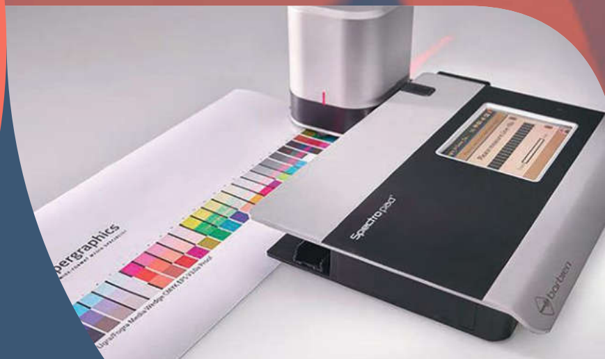
One of the most successful and popular standards is ISO 12647-7, the standard for contract proofs. Here a control strip measured using the spectrophotometer Spectropad from Barbieri.
