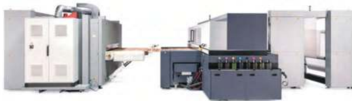
Durst Alpha Series 5 multi-pass inkjet press runs, acid, reactive and pigment ink formulations. The Alpha 190 can print at a maximum speed of 620 linear metres per hour.
