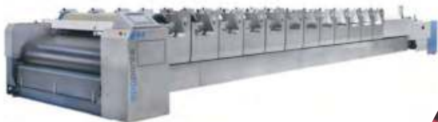
SPGPrints Pegasus EVO 12 colour rotary textile screen printing press capable of printing at 120 metres per minute at 2250mm wide.
